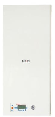
All of our boilers work on 12kw, requiring 50Amps, 10mm TW&E cable, 63 Amps RCD with 63 Amps Isolator.
